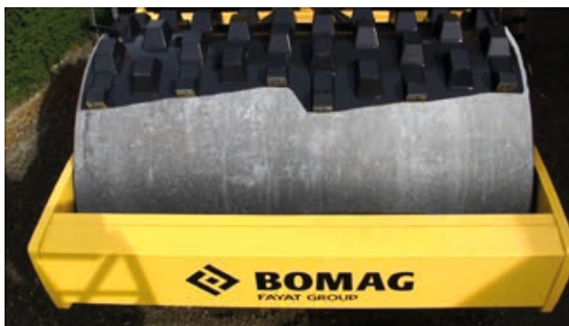
Quick changeover from smooth drum to padfoot drum for flexible working.
